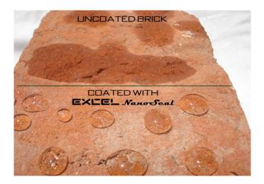
Hydrophobic coating can be applied to the bricks underlying the hard strata in the formation of foundation where ground water can prove to be harmful agent. Houses made up of brick masonry can be coated with hydrophobic coating so as to prevent the bricks from environmental pollution and natural calamities. To minimize the loss of water from wells or ponds, the bricks used can be coated and water absorption by bricks can be minimized.
