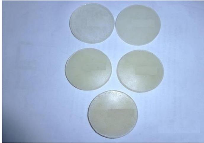
Fig. 3.7 Short glass fiber reinforced epoxy composites
