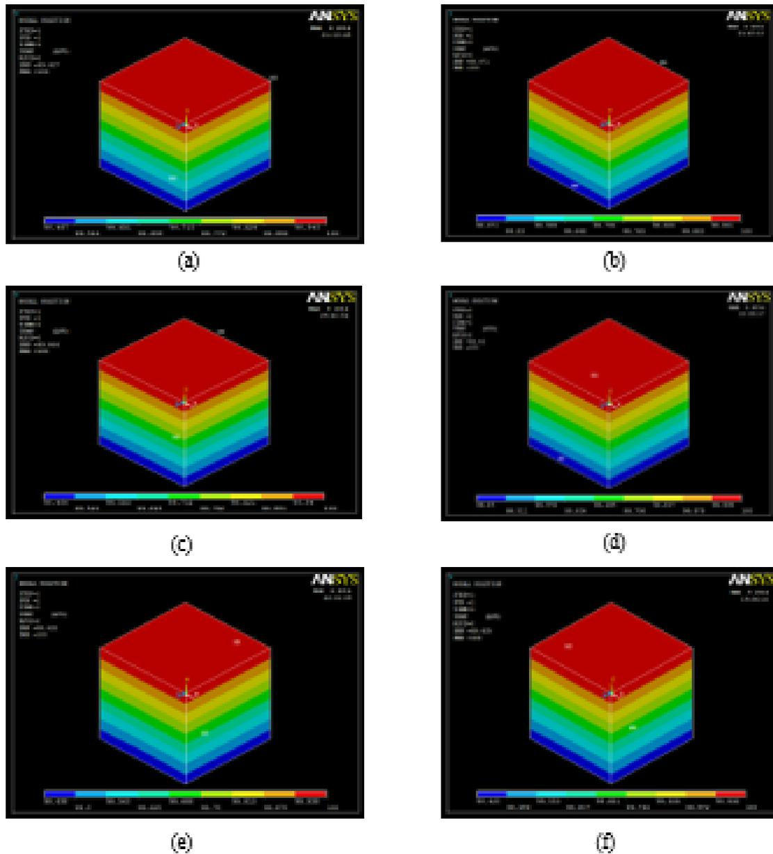
Fig. 4.4 Temperature profile of composites with banana fiber loading of (a) 2.83 vol% (b) 5.65 vol% (c) 7.54 vol% (d) 10.05 vol% (e) 12.56 vol% (f) 15.7 vol%
