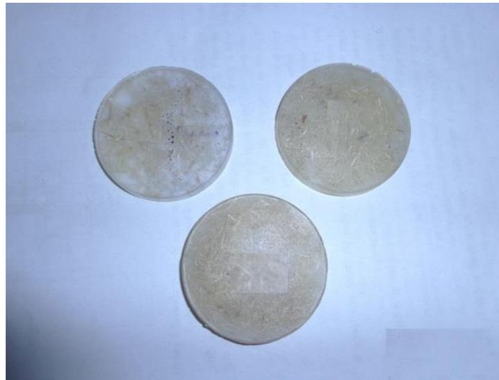
Fig. 3.8 Short banana fiber reinforced epoxy composites
