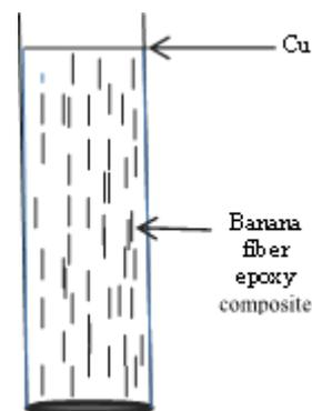
Fig. 3.6 Fiber reinforced epoxy composite fabrication by hand lay-up process
