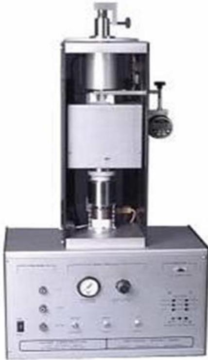
Fig. 3.8 Determination of Thermal Conductivity Using Unitherm™ Model 2022
