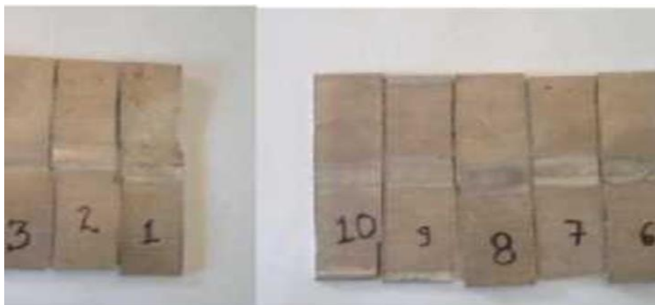
Figure 4 - a) Welded specimen performed with welding speed 3mm/s and welding current 100. 105, 110. 120 and 130A for samples numbers 1 to 5
