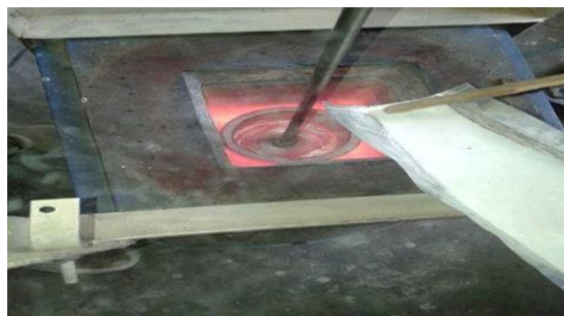
Figure 5.3 Preparation of sample by mechanical stir casting
