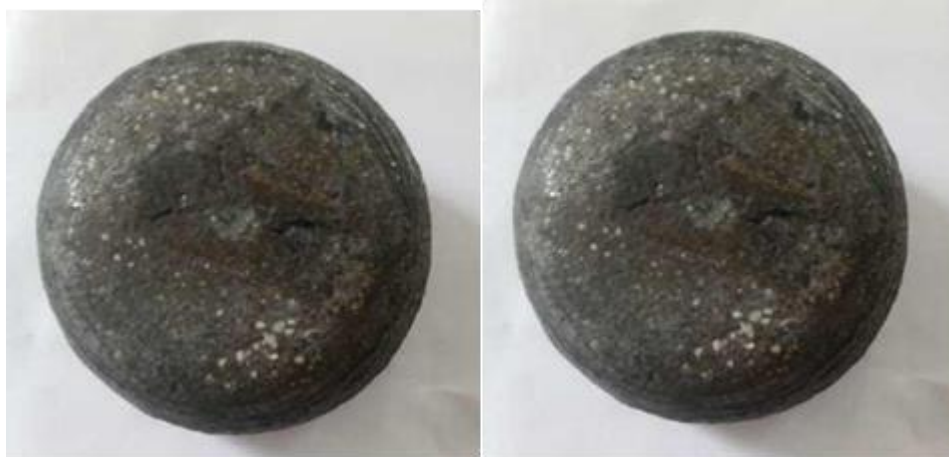
Figure 5.1 Sample of aluminium + Al 2 O 3 2.5 and 5% Alumina in Aluminium
