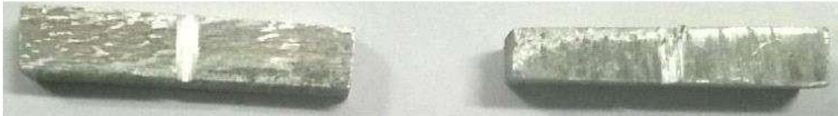
Fig 6.6 Toughness sample of 10% of Alumina in aluminum
