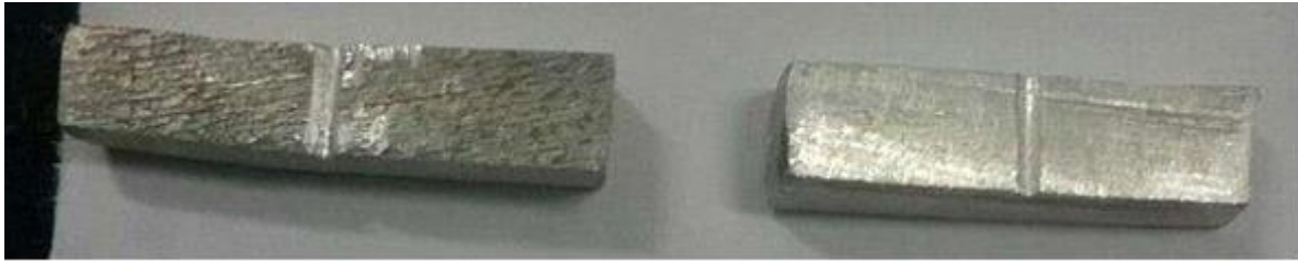
Fig 6.4 Toughness sample of 5% of Alumina in aluminum
