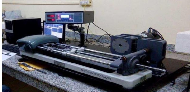
Fig. 6.2. Tensile Testing on Tensometer
