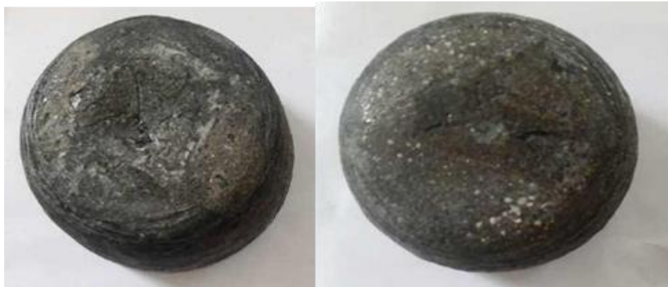
Figure 5.1 Sample of aluminium + Al 2 O 3 2.5 and 5% Alumina in Aluminium
