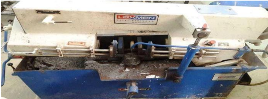
Figure 5.4 Cutting of samples on Power Hacksaw
