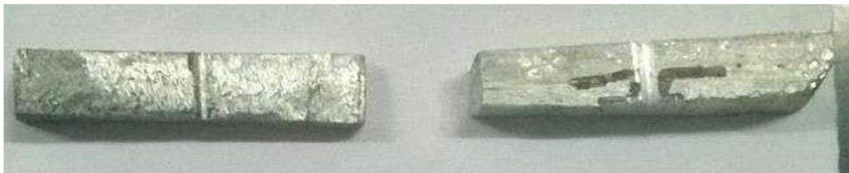
Fig 6.3 Toughness sample of 2.5 % of Alumina in aluminum
