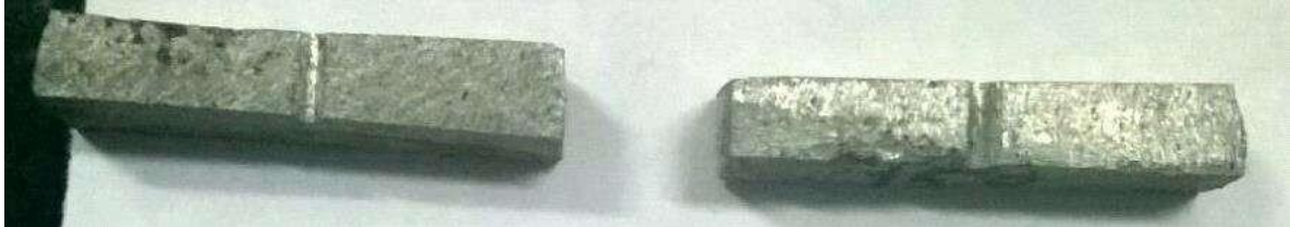
Fig. 6.5 Toughness sample of 7.5 % of Alumina in aluminum
