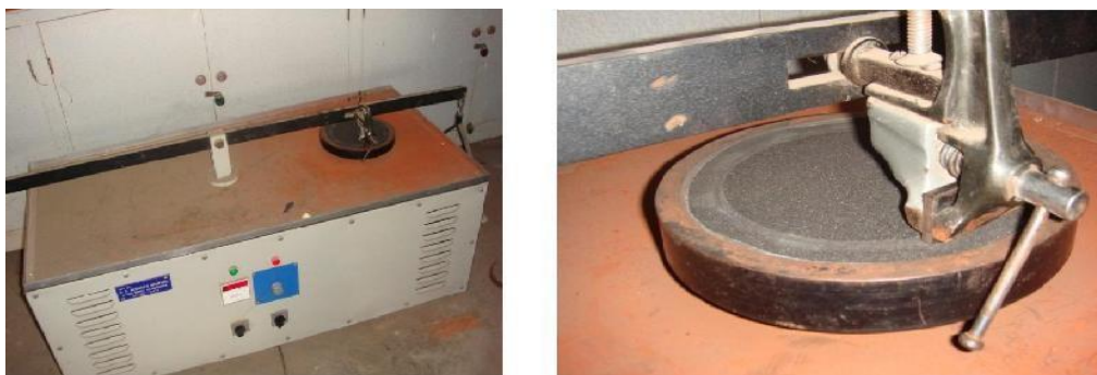
Fig. 2 Pin on disc machine for abrasive wear testing
