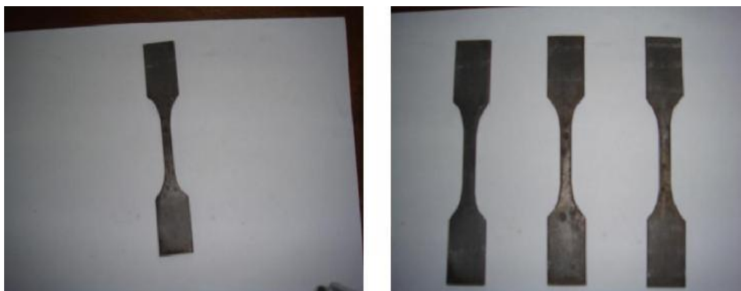
Fig. 5 Specimen for toughness test
