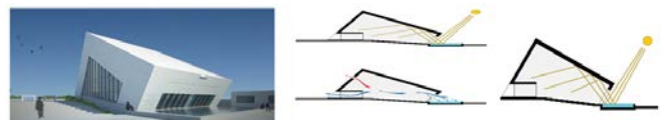
Fig. 19. Shows the effect of mass formation in natural lighting and natural ventilation [33].
