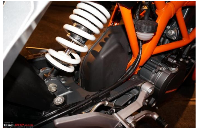
Fig 6 shock absorber in KTM DUKE 200
