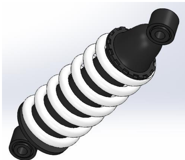
Fig 5 3-D modelling of KTM DUKE 200 shock absorber
