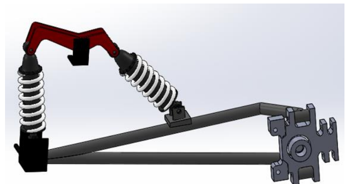
Fig 4 3-D modelling of rear suspension system with lever
