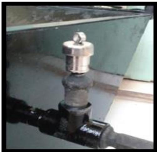
Safety valve use for the safety of the glass material of the system. Because the top side of insulation box is made with plane glass plate and also insulation box is assembled with the evacuated tubes.
