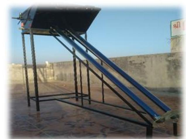
And also valves and T-section piping joint are provided on the adjacent of inclined plane for pouring water inside and extracting the hot water outside. And both boxes are assembled together and between them glass wool is provided for heating resisting purpose (Maintain inside temperature).
