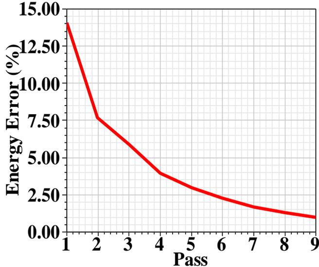
Figure 5: Energy Error (%) versus Adaptive Solution Pass
