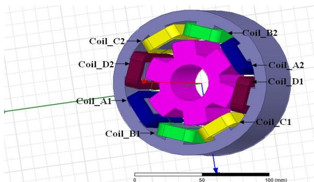
Figure 1: 4 Phase-8 Poles SRM Layout
