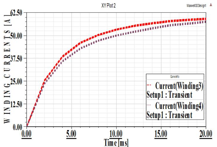
Figure 10: Winding3 and Winding4 Currents with Time
