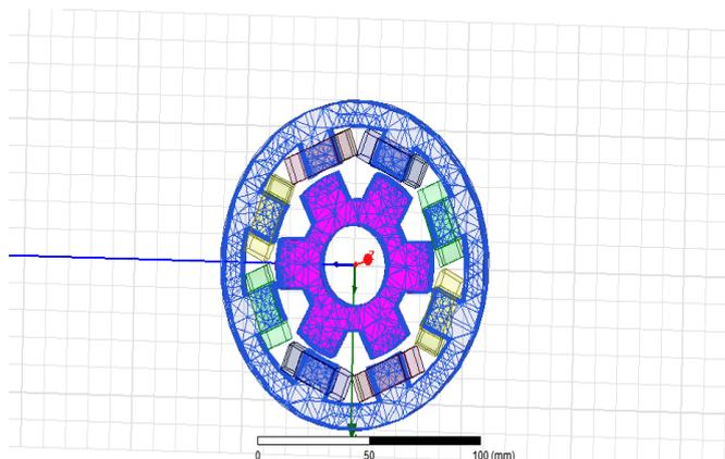
Figure 3: Finite Element Mesh of the SRM
