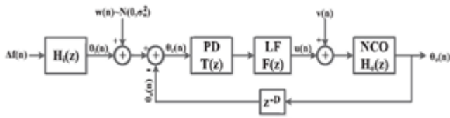
Fig3. Modeling of carrier recovery loop
