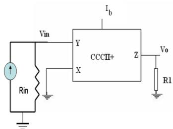
Fig.6 Circuit of Tunable Current Amplifier
