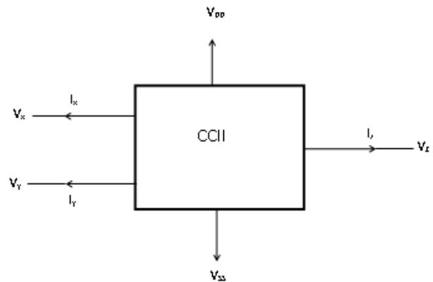
Fig.1 Current Conveyor Symbol and Characteristic
