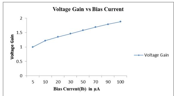
Fig. 9. Graph between Voltage Gain & Bias Current,  $R_1=1\text{K}$  constant
