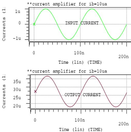
Fig. 7 Transient analysis for current amplifier
