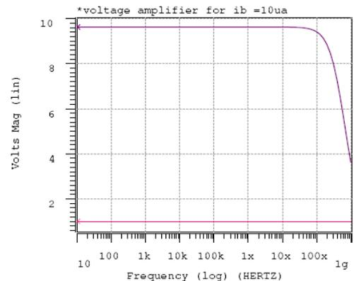
Fig.5 Frequency Response of Amplifier
