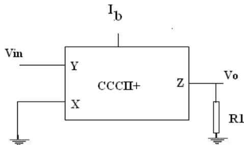
Fig.3 Circuit of Tunable Voltage Amplifier
