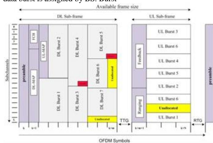
Fig. 1 TDD frame structure of mobile WiMAX.
