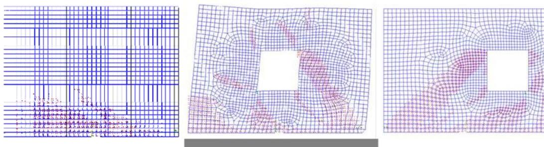
Figure 12. Crack patterns of the three analysed panel models
