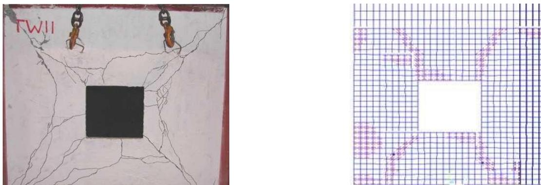
Figure 10. Experimental shear wall and ANSYS results
