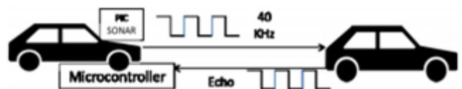
Fig. 2 Communication between Vehicles Using Sonar Pulse
