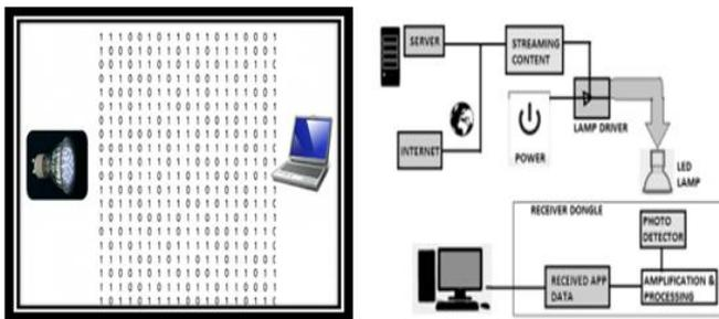
Fig3. Working Principle of Li-Fi
