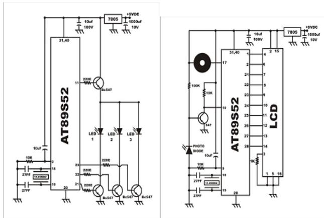
Fig 8 Interfacing diagram of VLC Transmitter and Receiver
