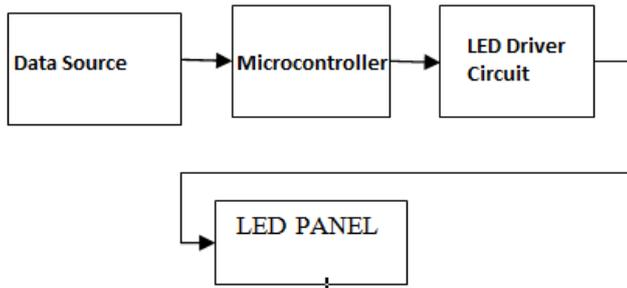
Fig. 6 VLC Transmission Part
