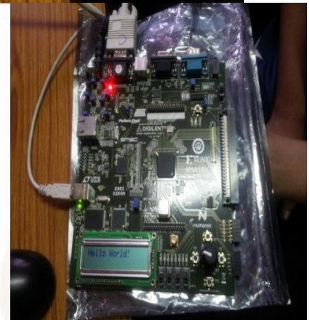
Figure 5. LCD Display “HELLO WORLD” Interfacing on FPGA
