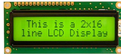
Figure 1.A 2 line x 16 characters LCD module[9]
