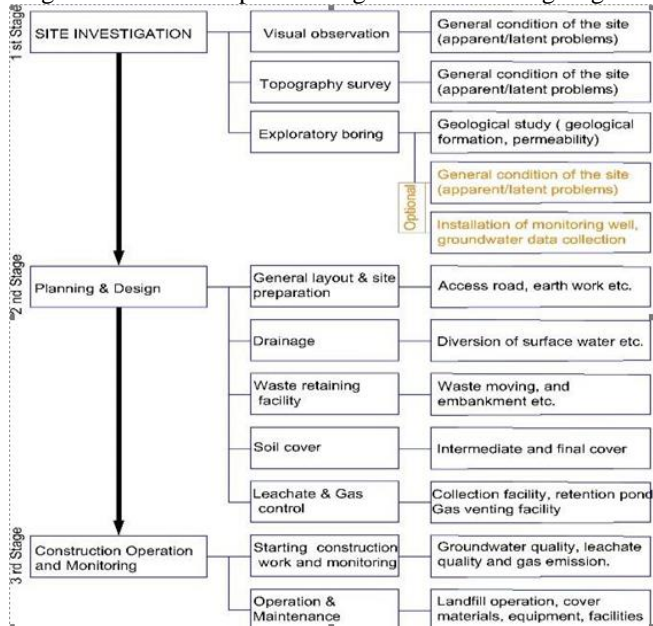
Fig 8. Flow process of landfill upgrading work [7]
