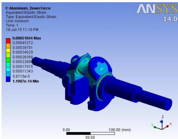
Fig. 6 Equivalent elastic strain of Al 5083 alloy Composite Crankshaft
