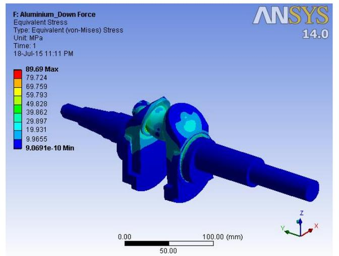
Fig. .4 Von Mises Stress of Al 5083 alloy Composite Crankshaft
