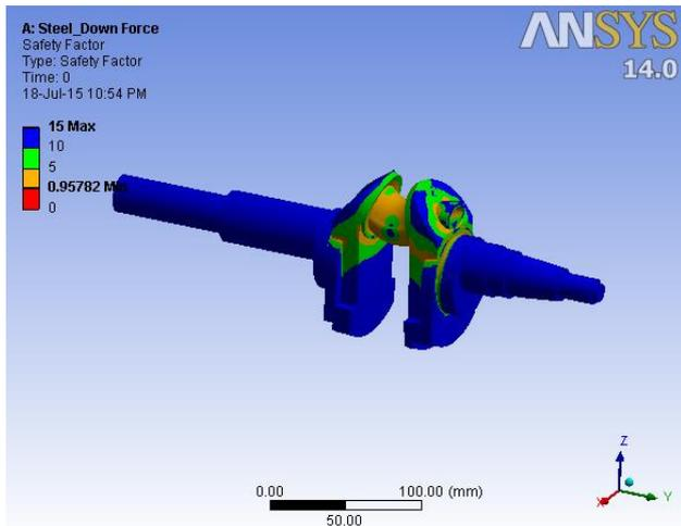
Fig.11 Safety Factor for Steel
