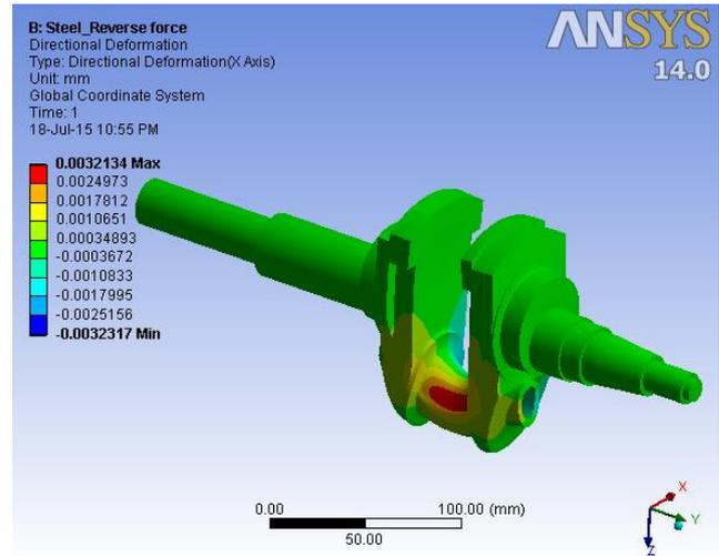
Fig.7 Total Deformation of Structure steel Crankshaft
