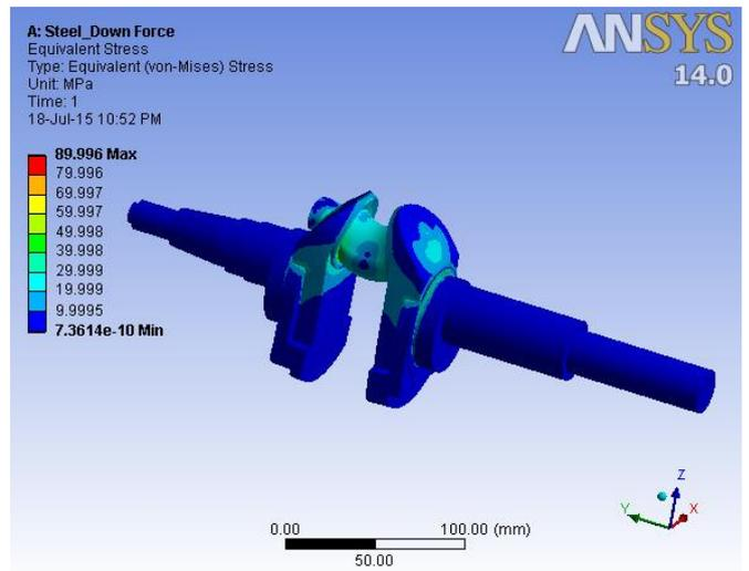
Fig. 3. VonMises Stress of Structural steel crankshaft
