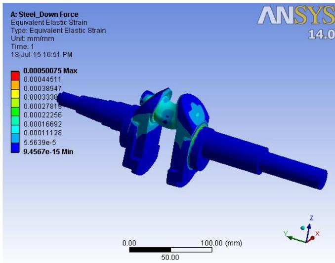
Fig. 5 Equivalent elastic strain of Structural steel crankshaft
