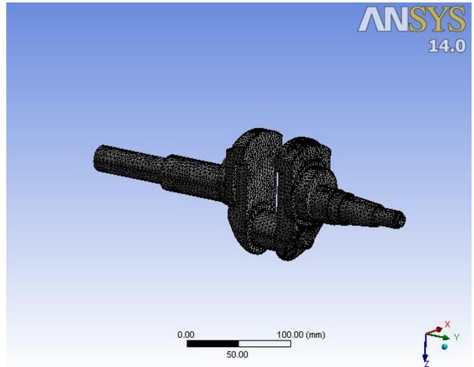
Fig.2 Meshed Model of Crankshaft
