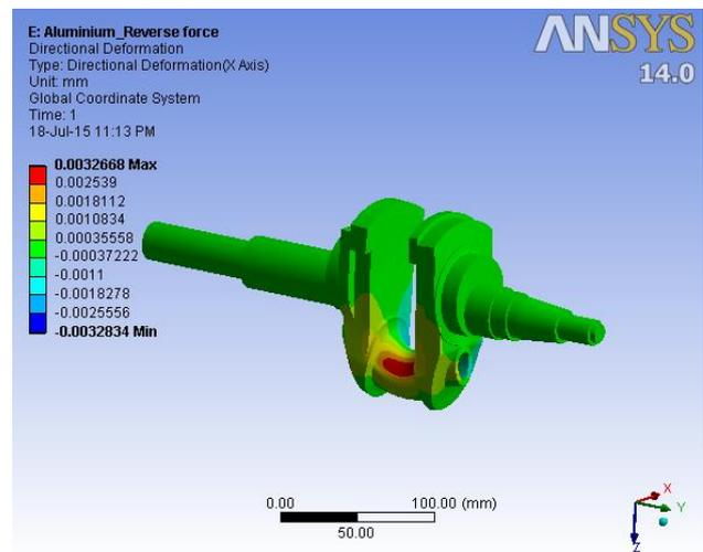
Fig.8 Total Deformation of Al 5083 Composite Crankshaft
