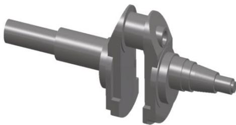
Fig 1-Solid Modelling of Crankshaft
