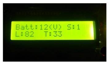
Fig. 2. LCD Screen showing battery voltage (Batt), timer (S), light intensity (L) and thermistor reading (T), clockwise from top
