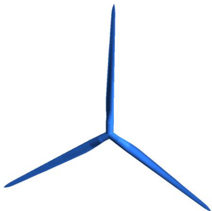
VI. FIG. 6. NREL 5MW ROTOR WITH THE BLADE ROOTS EXTENDED AT THE HUB CENTER
