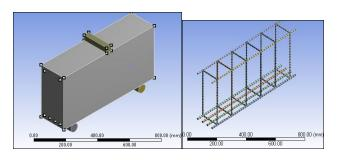
Fig. 4. Modelling of deep beam in ANSYS
